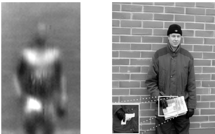
Fig. 3. A millimeter wave image and a photo of a person carrying a handgun silhouette inside the newspaper.
