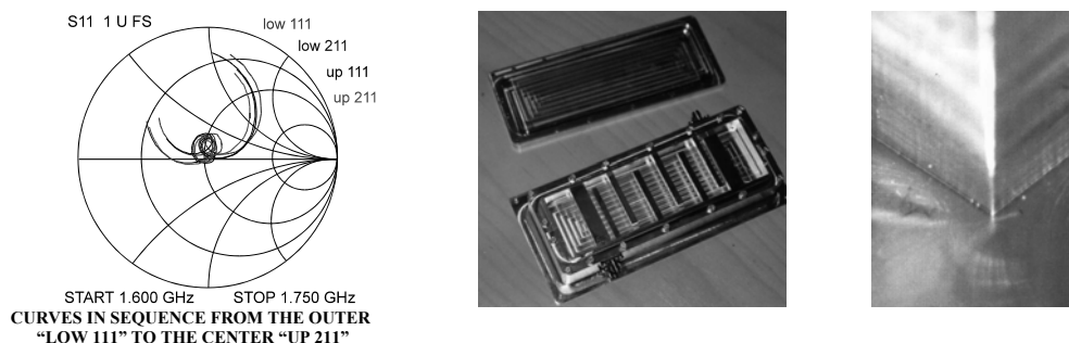
Fig. 3. The Smith chart presentation of S11 shows that the two filters with ultimately sharp resonator roots give a good impedance match over the entire pass band (left). The track of the milling tool is visible on the bottom. Surface roughness is 0.8 \mu\text{m} (middle). A photo of the resonator root, which width is 5 mm (right) [2] and [5].
