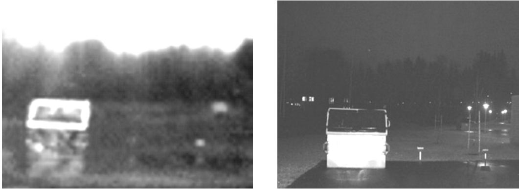
Fig. 4. A millimeter wave image and a photo of a night time scenery.
