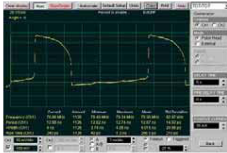
Figure 4. Measured curveforms of the TD- oscillator circuit.
